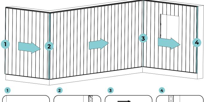
Begin by fixing the corner profile into place before installing the first board.
