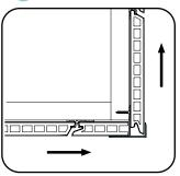
Affix the corner profile after the last board on this wall has been installed.
