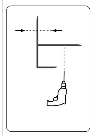
The multi-functional corner profile can have holes drilled into it in different places, depending on how it is used on the cladding.
