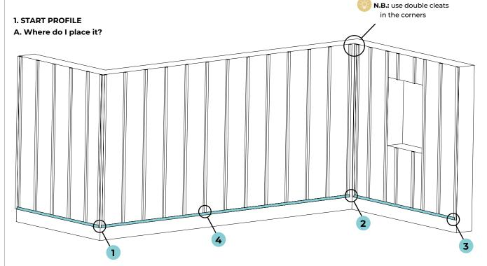
When positioning the start profiles, maintain the distances specified below in order to leave room for the multi-functional corner profile.
