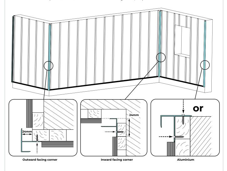
To position the corner profile correctly, use the low groove of the start profile as a marker.
