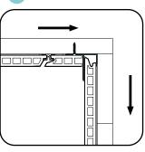
Affix the corner profile before installing the last board on this wall. Then fix the board in place using a Silvadec® special composite screw.
