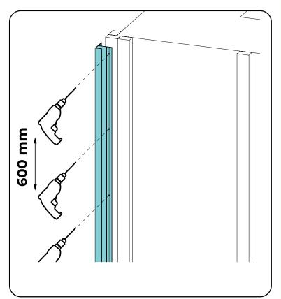
Drill into the groove of the profile, then screw the profile onto the cleat, leaving a gap of 600 mm between adjacent screws.
