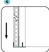
To finish with a corner profile, fix this profile in place after the final board.
