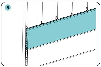
6. Fix each board in place using fastening clips, screwing these into place where each board meets a cleat.
