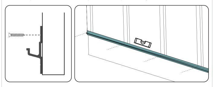
To prevent water pooling in the slot of the profile, drill a hole with diameter between  $\emptyset$  3 mm and  $\emptyset$  5 mm at the point where the board ends will meet. (for horizontal installation only).
